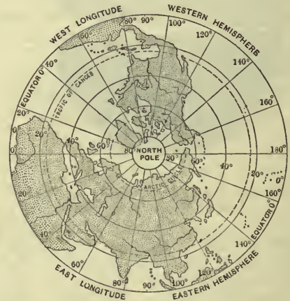
FIG. 687.—A view looking down on the north pole, to show how the meridians come to a point at the north pole. Notice that if the 0^{\circ} meridian were continued, it would unite with the meridian 180^{\circ} .
